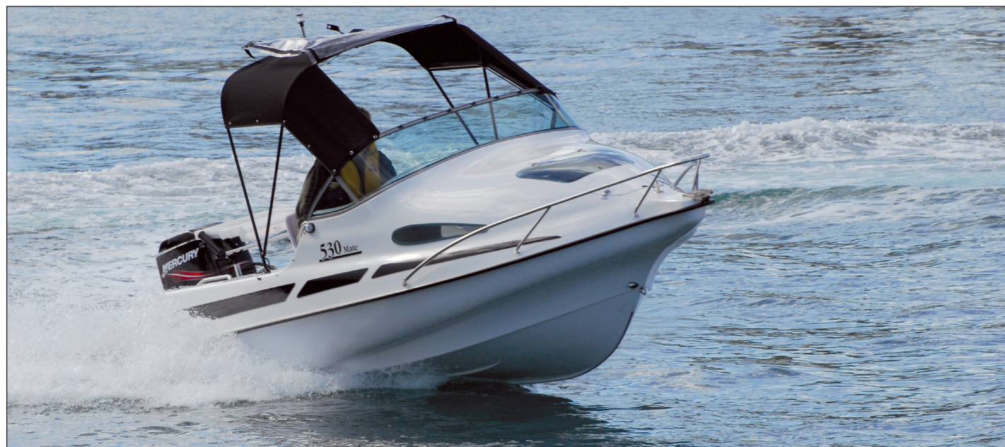
ABOVE AND BELOW: These photos clearly illustrate the way the water is turned down and how it leaves the hull well astern. OPPOSITE: The angle of entrance contributes to the stability and dryness of the ride as well.
