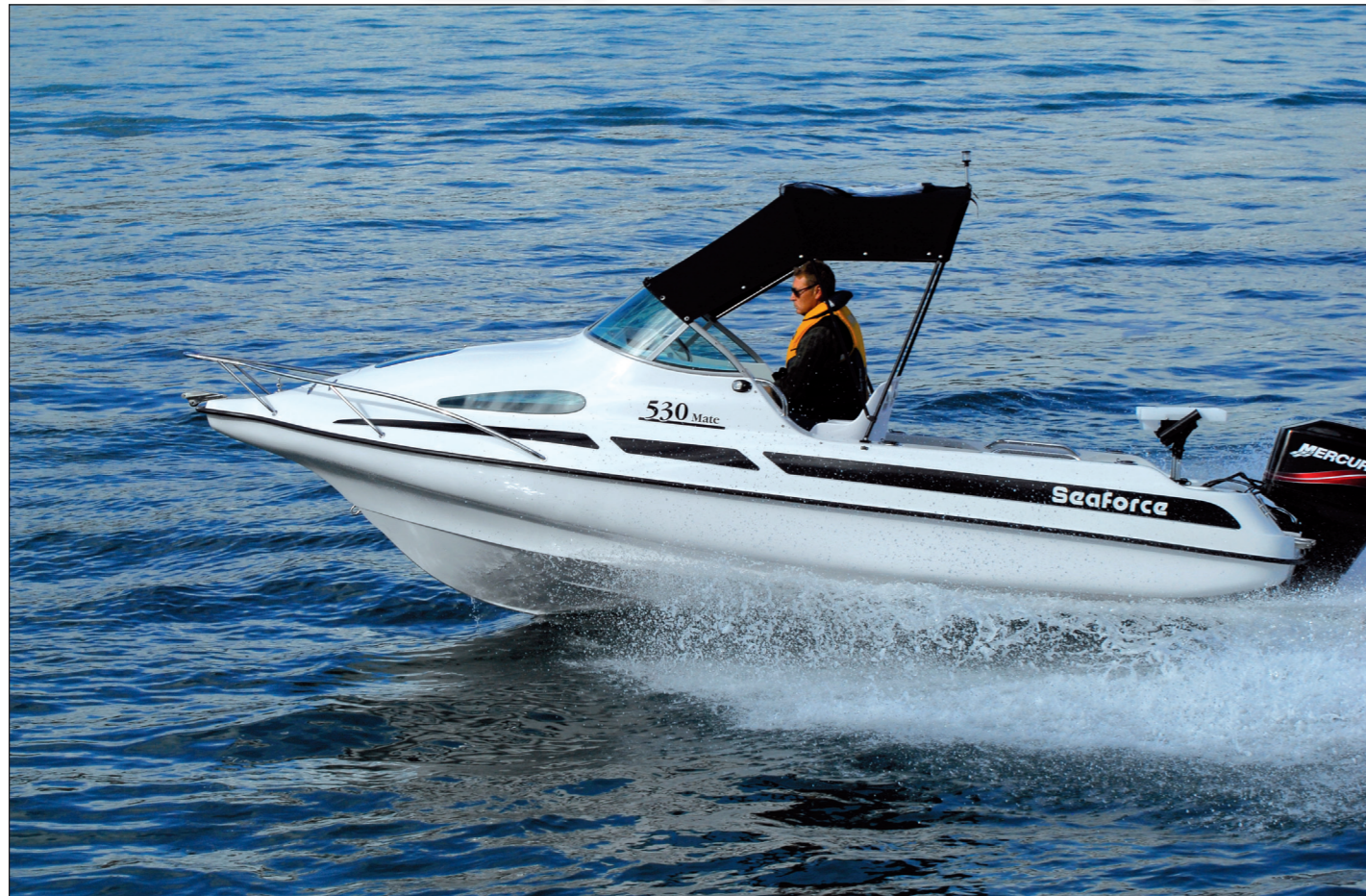
ABOVE AND BELOW: These photos clearly illustrate the way the water is turned down and how it leaves the hull well astern. OPPOSITE: The angle of entrance contributes to the stability and dryness of the ride as well.
